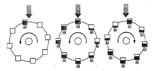
THE LORENZIAN WATERWHEEL. The first, famous chaotic system discovered by Edward Lorenz corresponds exactly to a mechanical device: a waterwheel. This simple device proves capable of surprisingly complicated behavior.
